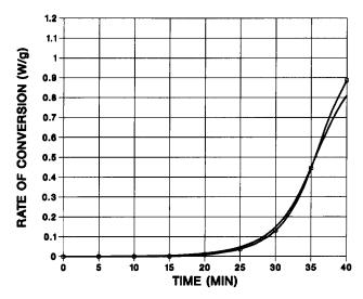
Figure 3 Verification of conversion kinetic model for dynamic heating: —, Cole's model; —O—, experimental data
