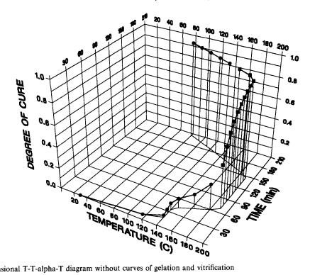
Figure 8 Three-dimensional T-T-alpha-T diagram without curves of gelation and vitrification
