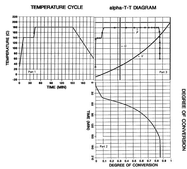
Figure 6 Three-part alpha-T-T diagram
