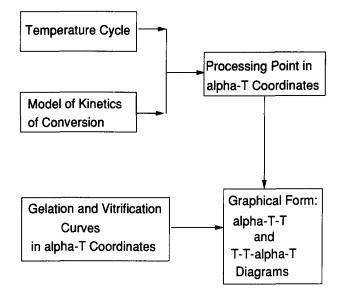
Figure 1 Structure of the system
