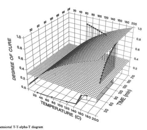
Figure 7 Three-dimensional T-T-alpha-T diagram
