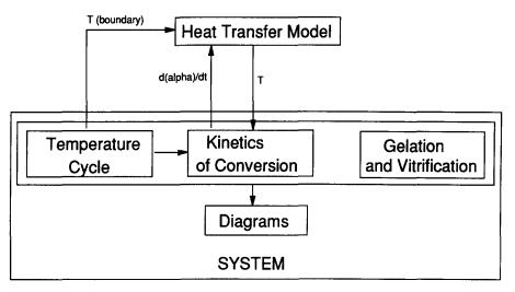
Figure 2 Interaction of the proposed system with composite processing model
