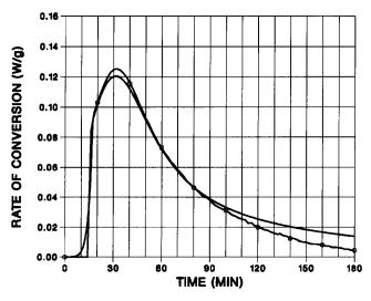
Figure 4 Verification of conversion kinetic model for isothermal heating: —, Cole's model; —O—, experimental data
