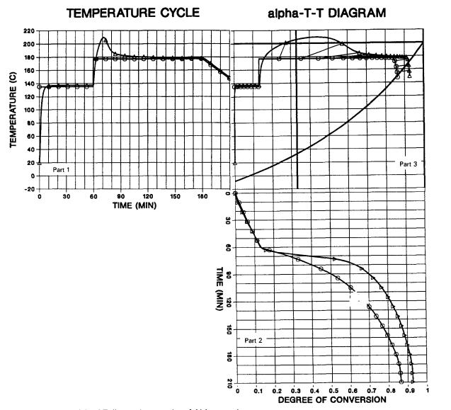
Figure 9 Three-part alpha-T-T diagram in processing of thick composites
